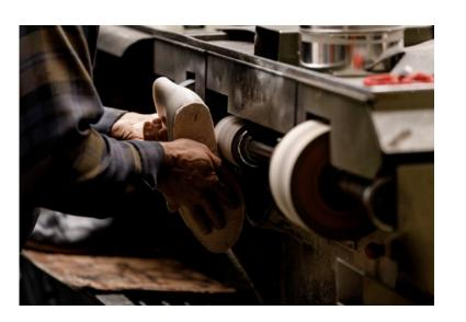
Top: Before trimming the leather insole with a blade, Shafee attaches it to a last with three temporary nails. Bottom: He sands the insole to more precisely match the shape of the last.
